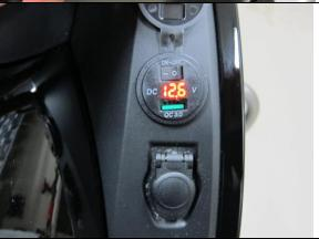
For connection to the accessory power socket, connect the supplied harness to the USB (red = + / brown = -). Remove the Hirschmann connector from the existing accessory power socket and connect that lead to the mating plug on the "Y" harness at right. Connect the other mating "Y" harness plug to the accessory power socket. With this connection, the socket should shut-off 50 seconds after ignition-OFF.
